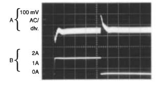
Horizontal Time Base: 100 μs/div. A: Output Voltage, 100 mV/div. (AC) B: 500 mA to 2A Load Pulse
